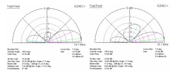
The model SWR on 20 m is still good BUT the SWR on 17m is sadly well above 2 even after fiddling with the 17 m dimensions in the model. The good news is that I have a KAT500 tuner to overcome that SWR issue. So let's give it a go.
