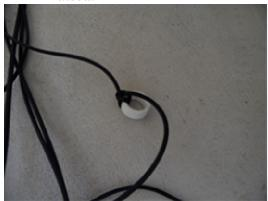
This produces, with some fiddling with wire lengths, an impedance around 20 - j20 which can be matched using a practical "hairpin" coil shunt of inductive reactance ~ 45 ohms (4 microHenrys, say 5 turns 4" dia).
